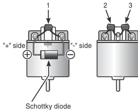
Motors with no suppressor capacitors, or inadequate suppression, may cause the receiver to malfunction. Always solder the capacitors supplied to your motor.
