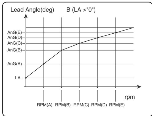
When using in races in which the lead angle setting function is inhibited by the ESC, set LAU (LEAD ANGLE USE) to OFF. The LAU setting has priority over TBM-(TURBO MODE). If LAU is set to "OFF", the lead angle setting function can be turned off even if TBM is set to "LV1" or "LV2".
