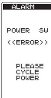
If the power switch is quickly switched from the DISP mode to the PW ON mode or vice versa, the switch error shown at the left may be generated. If this occurs, cycle the power.
