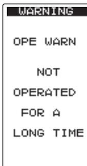
If the T4PL is not operated for 10 minutes, an audible alarm is sounded and "OPE WARN" is displayed on the screen. The audible alarm stops when the steering wheel, throttle trigger, and any dial, switch, or edit button is operated. If you are not going to use the transmitter, turn the power off. (Setting can be reset at the system menu on page 93.)
