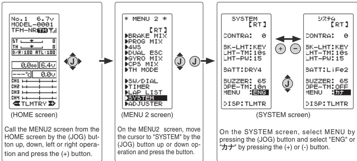
After changing the setting, return to the MENU2 screen by pressing the (JOG) button or return to the HOME screen by selecting [RT] and pressing the (JOG) button.
