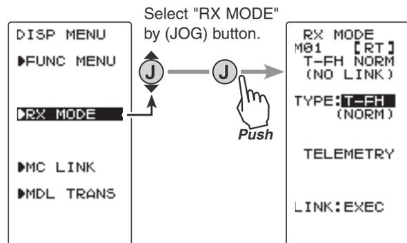
**2** Move the cursor to "TYPE: ----" by (JOG) button up or down operation, and select the RX type with the (+) button or (-) button.
