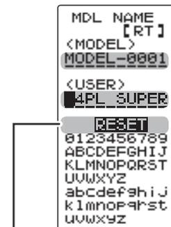
Move the cursor to "RESET" by the (JOG) button up or down operation.
