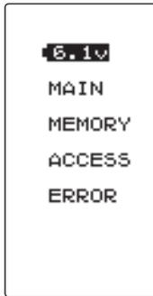
If the data in the transmitter is not transferred normally when the power is turned on, an audible alarm will sound and "MAIN MEMORY ACCESS ERROR" will be displayed on the LCD.
