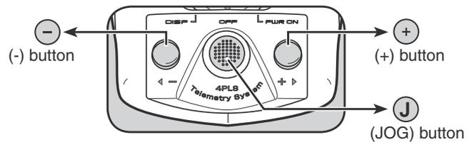
**1** Set the transmitter power switch to DISP. Select "RX Setting" by (JOG) button up or down operation, and display the "RX MODE" screen by pressing the (JOG) button.
