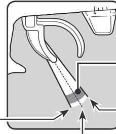
Position at which motor starts to run
