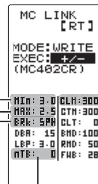
"Min" which sets the frequency when the load is small, is set to the high frequency side (large value) when extension is desired after straight-aways and curves.
