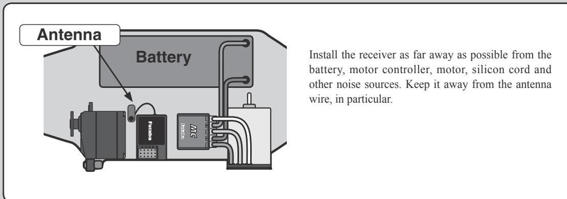
Install the receiver as far away as possible from the battery, motor controller, motor, silicon cord and other noise sources. Keep it away from the antenna wire, in particular.
