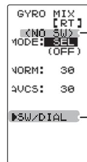
The function select switch screen (P65) can be displayed from this screen.
