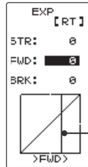
Vertical cursor moves in step with throttle trigger operation.
