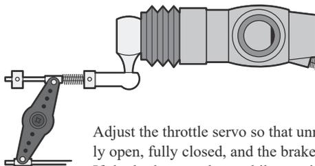
Adjust the throttle servo so that unreasonable force is not applied when the engine carburetor is fully open, fully closed, and the brakes are applied fully.
