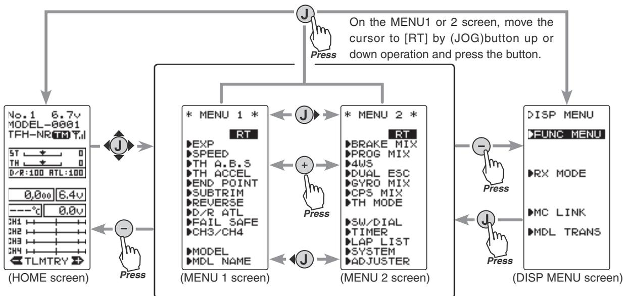
On the DISP MENU screen, move the cursor to "FUNC MENU" by (JOG) button up or down operation and press the button.
