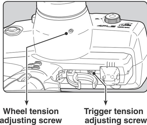
**Wheel tension adjusting screw**
