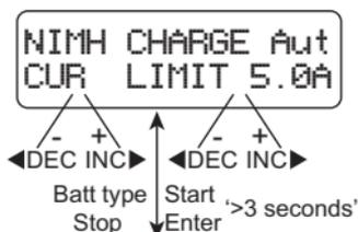
This program is for charging of NiCd/NiMH batteries associated with R/C models applications. You can press START/ENTER key to make it blink and then INC or DEC to change the parameter value. Press START/ENTER key to store the value.
