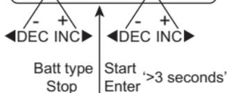
The value of discharge current on the left can not exceed 1C, and the value on the right can not be under the voltage recommended by the manufacturer to avoid deep discharging. Press START/ENTER for more than 3 seconds to start discharging.
