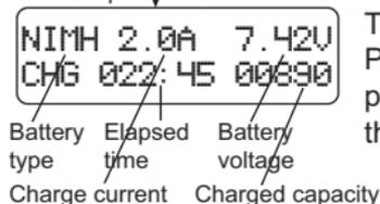
The screen shows the real-time status. Press BATT TYPE/STOP key to end the program. The sound will emitted to indicates the end of program.
