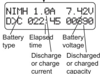
Press BATT TYPE/STOP key to stop program, you can press START/ENTER key to alter charge current. The sound indicates the end of program.
