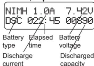
The screen indicates the discharging state. You can press START/ENTER key to alter discharge current. Press START/ENTER again to store the value. Press BATT TYPE/STOP key to stop discharging. The emitted sound alerts the end of discharging.
