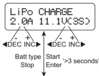
The left side of the first line shows the type of battery you choose. The value on the left of the second line of the charger is current user set, After setting the current and voltage, press START/ENTER key for more than 3 seconds to start the process.(charge current: 0.1-5.0A, voltage: 3.7-22.2V).
