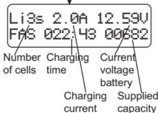
This screen shows the real-time status during charge process. Press BATT TYPE/STOP key once to stop the charge process.
