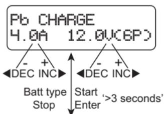
Set up the charge current on the left and nominal voltage on the right. Range of current is 0.1-5.0A, the voltage should match the battery being charged. Press START/ENTER key for more than 3 seconds to start charging.
