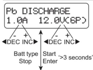
Set up the charge current on the left and nominal voltage on the right. Range of discharge current is 0.1-1.0A, the voltage should match the battery being charged. Press START/ENTER key for more than 3 seconds to start charging.
