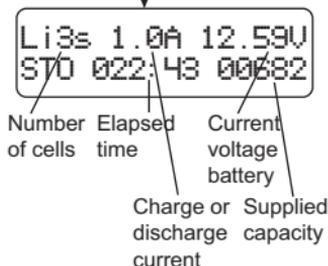
This screen shows the real-time status charging. Press BATT TYPE/STOP key once to stop the charge process.
