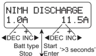
Set charge current on the left and the final voltage on the right. Range of the charge current is 0.1-1.0A; range of final voltage is 0.1-25.0V. Press START/ENTER key for more than 3 seconds to start the program.
