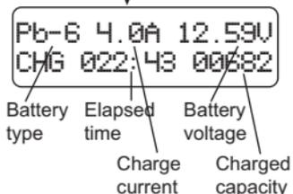
The screen displays the real-time discharging status. Press START/ENTER key to alter discharge current. Press START/ENTER key again to store the parameter value you set. Press BATT TYPE/STOP key to end the program.
