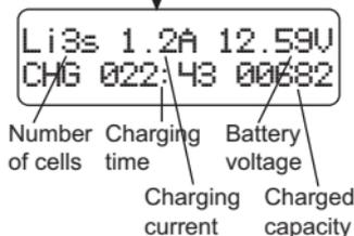
This screen shows the real-time status during charge process. Press BATT TYPE/ STOP key once to stop the charge process.
