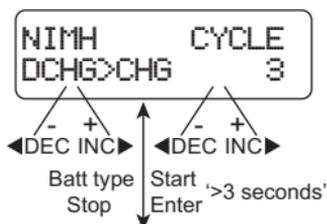
You can set up sequence on the left and the number of cycles on the right. Range of the cycle number is 1-5.
