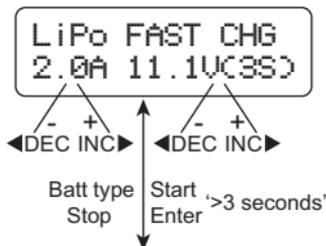
The value on the left side of the second lines sets the charge current. The value on the right side of the second lines sets the battery pack's voltage. After setting current and voltage, press STAR/ENTER for more than 3 seconds to start the process.
