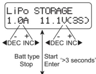
At this screen, you can set up the current and voltage of the battery pack. Charging and discharging will make the batteries come to the voltage level of "Storage" state.
